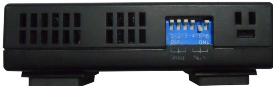
Figure 8-6 Temperature sensor DIP switch settings
