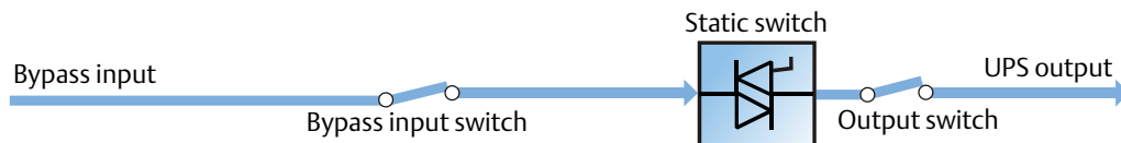
Figure 1-5 Bypass operating mode line diagram
