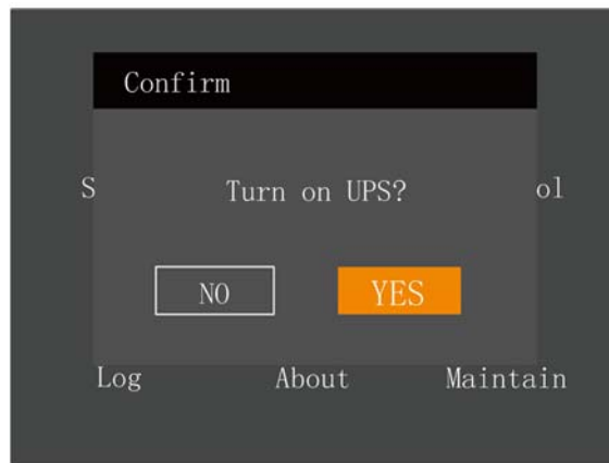
Figure 5-5 Switching the UPS on
