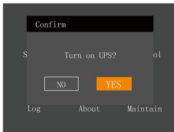
Figure 5-7 Switching the UPS on
