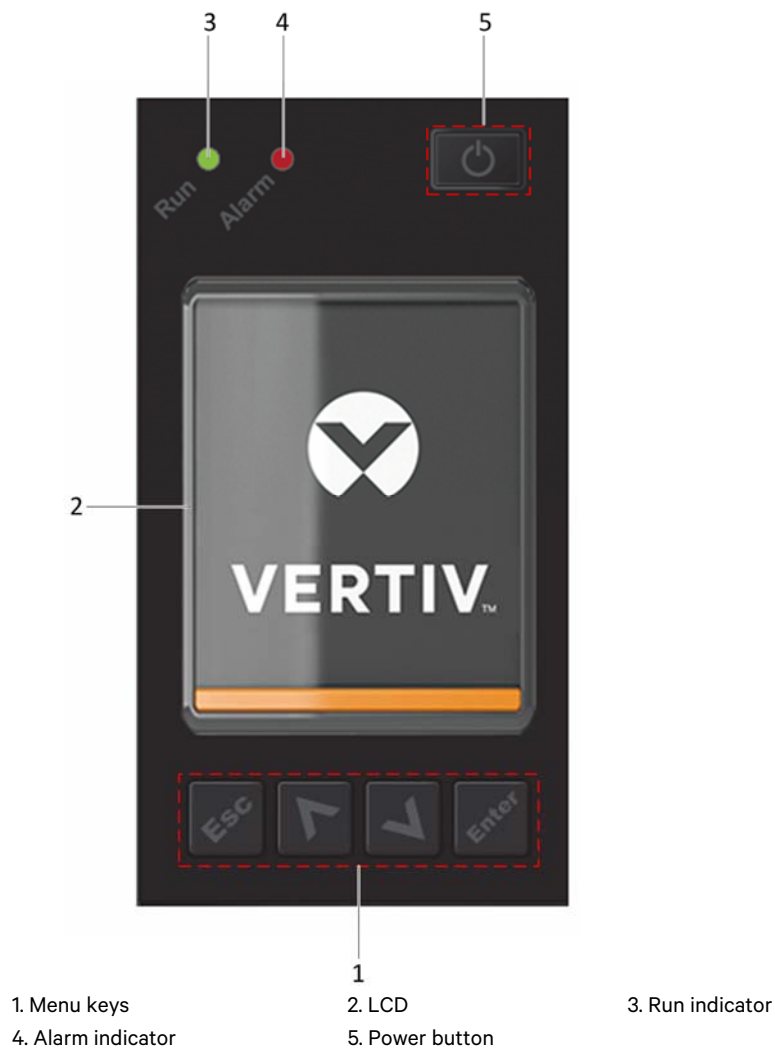
Figure 4-1 Operation and display panel
